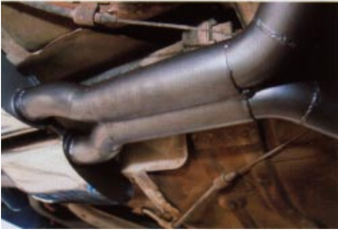
The big, 10-inch X-pipe proved to be the most effective of the two different combinations
