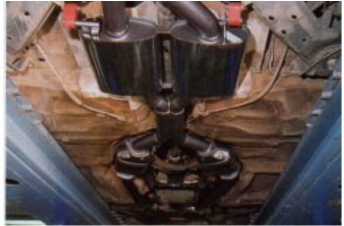
The system uses twin GM catalytic converters and twin straight-through mufflers
