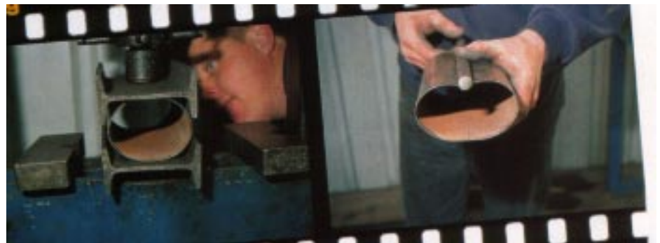
The 5-inch pipe was first pressed to the right height then ... a rod was used to form the shape
