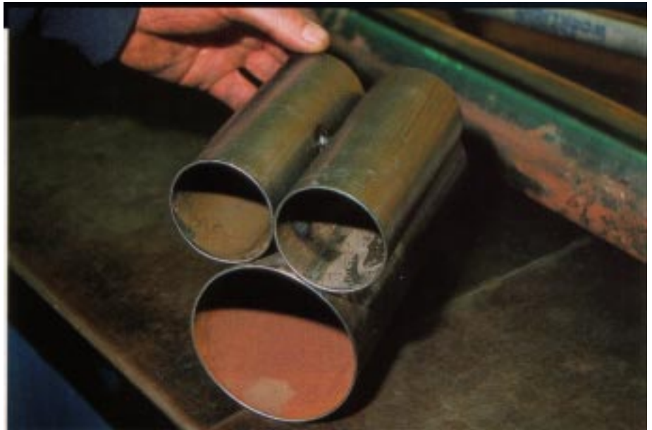
The initial problem was how to fit these twin pipes into a 5-inch pipe to make the X system
